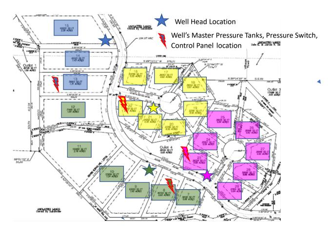
The AREF Phase I Shared Well System is a private water system serving AR Lots 7-29. All water available for these Phase I Lots is obtained from a series of wells that service individual cluster of lots. There are four wells located in AR Phase I supplying water between three to seven lots each. (see above) Well Control System (Master Pressure Tank, Pressure Switch, Control Panel) is located in one of the residences contained within each cluster.
